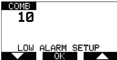
Fig. 8 Sensor Alarm Setup
