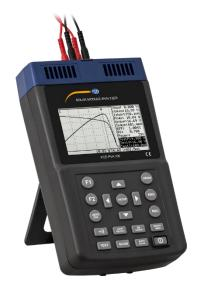
100 and a test solar module can also be used to determine the optimum values for the alignment and the angle of inclination of the modules.
