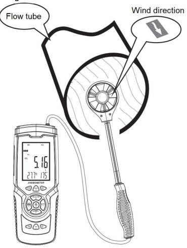
To make a measurement, align the flow sensor with the direction of the flow. An arrow on the head of the sensor indicates the orientation in relation to the wind flow. Wait for at least two seconds for the reading to stabilise.
