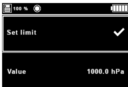
Fig. 58 Alert menu for pressure sensor
