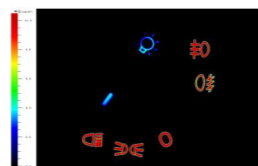
指示按键亮度均匀性测试 Luminance uniformity test for keyboard
