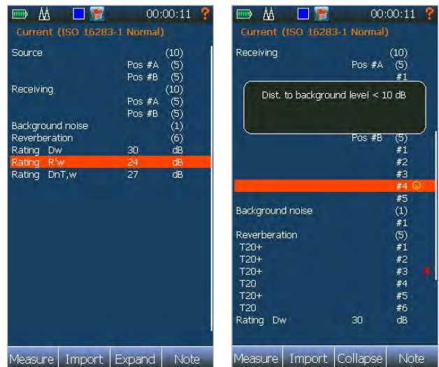
Project View display an overview of the entire measurement project in a concentrated form (left) and with all details in the expanded form (right)
