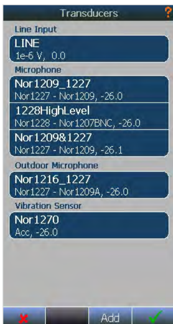
The Transducers menu The calibration history gives you full traceability of the microphone sensitivity.
