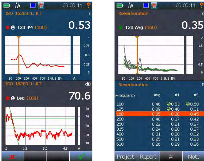
Graphical Reverberation Decay (left). Move with the cursor along the frequency axis to display the corresponding graphical reverberation curve. Press the Num button to get the corresponding numerical values. Alternatively, all reverberation time measurements and the average values are displayed together (right).
