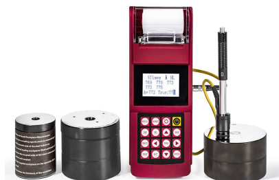
Calibration on HLD/HRC/HB Blocks
