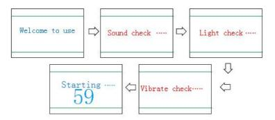
After self-check is done, the device enters into detection interface (see below).
