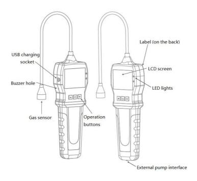
2.2 Structure: the main shell, circuit boards, batteries, display, sensors, chargers.
