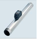
testo 6453 compressed air meter including inflow/outflow section, diameter DN40 (11/2"), analog output and integrated pressure measurement \*
