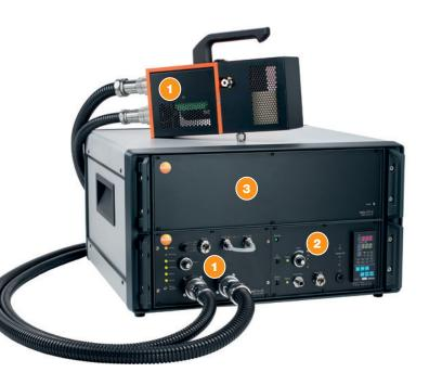
Hot dilution is carried out with Testo's rotating disk diluter testo MD19-3E 1. The combination of a rotating disk diluter, an air supply evaporation tube – testo ASET15-1 2 and a data acquisition unit testo CU-2 3 forms a complete ThermoDiluter system known as volatile particle remover testo ViPR.
