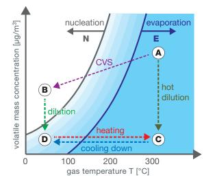
In a dilution tunnel both the concentration and the temperature of the substance are reduced ((A --> (B)). During dilution, the compound passes its dew point and nucleates into nanodroplets (curve N). Subsequent secondary dilution ((B --> (D)) will reduce the number concentration of the droplets, but is unable to evaporate them, because of a hysteresis effect between nucleation and evaporation.
