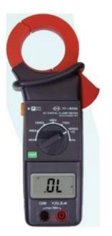
CAT III 1000V 3-3/4 digit LCD display with maximum reading of 4000. Overload indication. Low battery indication. AC voltage range: 0 to 750V. AC current range: 0 to 1000A. Peak Hold. Test Ranges: ACV, ACA, Resistance, Frequency, Continuity. Non-contact frequency measurement. Auto Power Off. Double Injection outer case.
