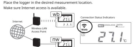
Press the <REC/STOP> button to immediately send the recorded data to "T&D WebStorage Service" without waiting for the next transmission. If the transmission is successful, Web will remain ON after COM turns OFF.
