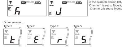
The factory default setting is "K" for both 1 2. Depending on the thermocouple type you're going to use, make settings or changes using "T&D WebStorage Service" or the software "TR7 for Windows".
