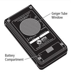
tube. The small radiation symbols on the front label (5) and the end label (9) indicate the center of the Geiger tube.
