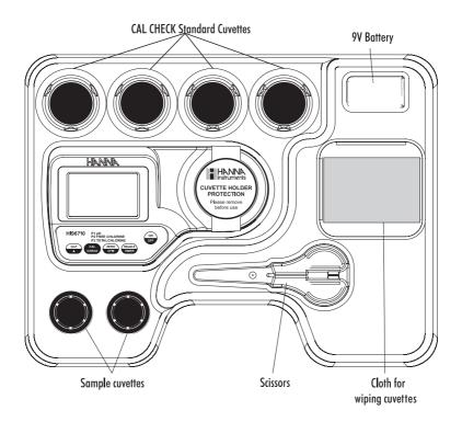
The H196710 is an auto diagnostic portable microprocessor meter that benefits from Hanna Instruments' years of experience as a manufacturer of analytical instruments. It has the advanced optical system based on a special tungsten lamp and a narrow band interference filter that allows most accurate and repeatable readings. All instruments are factory calibrated and the electronic and optical design minimizes the need of frequent calibration.
