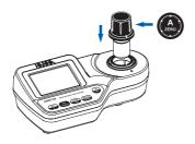
Press ZERO/CFM and the lamp, cuvette and detector icons will appear on the display, depending
