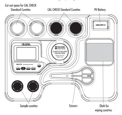
The H196709 is an auto diagnostic portable microprocessor meter that benefits from Hanna Instruments' years of experience as a manufacturer of analytical instruments. It has the advanced optical system based on a special tungsten lamp and a narrow band interference filter that allows most accurate and repeatable readings. All instruments are factory calibrated and the electronic and optical design minimizes the need of frequent calibration.
