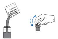
• Replace the cuvette into the holder and ensure that the notch on the cap is positioned securely into the groove.
