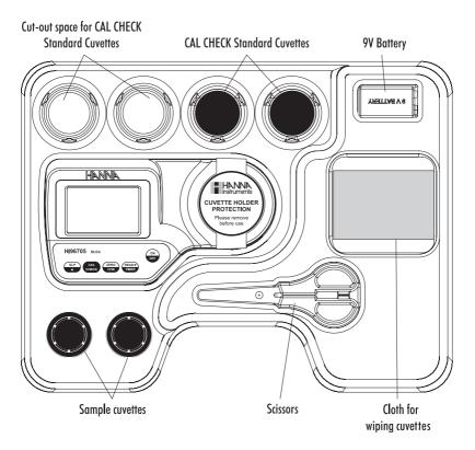
The H196705 is an auto diagnostic portable microprocessor meter that benefits from Hanna Instruments' years of experience as a manufacturer of analytical instruments. It has the advanced optical system based on a special Tungsten Lamp and a narrow band interference filter that allows most accurate and repeatable readings. All instruments are factory calibrated and the electronic and optical design minimizes the need of frequent calibration.
