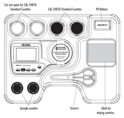
The H196701 is an auto diagnostic portable microprocessor meter that benefits from Hanna Instruments' years of experience as a manufacturer of analytical instruments. It has the advanced optical system based on a special tungsten lamp and a narrow band interference filter that allows most accurate and repeatable readings. All instruments are factory calibrated and the electronic and optical design minimizes the need of frequent calibration.
