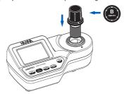
Press CAL CHECK and the lamp, cuvette and detector icons together with "CAL CHECK" will
