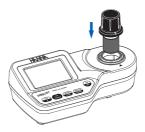
Press and hold READ >/TIMER for three seconds. The display will show the countdown prior to measurement. The beeper is playing a beep at the end of countdown period.
