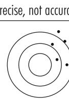
In a laboratory using a standard solution of 1.00 mg/L chlorine and a representative lot of reagent, an operator obtained with a single instrument a standard deviation of 0.02 mg/L.
