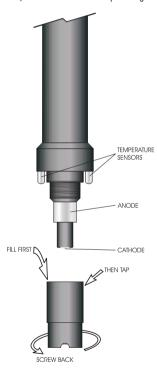
4. Whit the sensor facing down screw the cap clockwise to the end of the threads. Some electrolyte will overflow.
