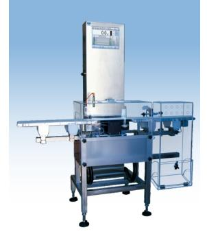
Automatic checkweigher DWM/WL/HP series is intended to weighing goods requiring the highest measuring accuracy. The checkweigher comprises an electromagnetic weighing module ensuring readability of 0,05g. The scale are mainly applicable in pharmaceutical plants, and chemical and food-processing industry.
