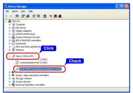
Check the COM number on the right of "HIOKI IM3570 Impedance Analyzer" port in the [Ports (COM & LPT)] list.
