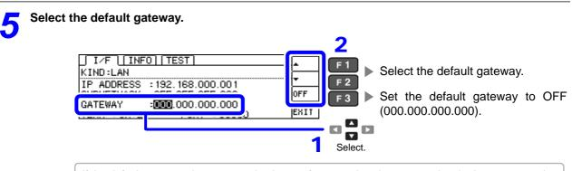
If the default gateway does not need to be set, for example, when connecting the instrument and computer on a one-to-one basis using a cross cable, leave this set to OFF.
