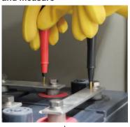
When the measured value stabilizes, save it automatically without having to operate the switch. Wait time can be as short as only 2 seconds to auto-save from when the test leads make contact with the battery terminals, cutting time by 60% compared to the legacy product.
