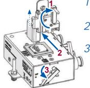
Turn the pusher up/down operation knob in the "up" direction to raise the tip pin.
