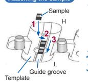
Place the sample on the template using a pair of tweezers. Align the sample's electrodes
