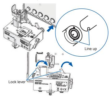
Adjust the adjustor so that the connector is not subject to excessive force.
