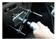
Tactile test of rotary switches on car dashboard
