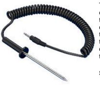
The 80PR 60 probe expands the utility of your RTD non-contact infrared thermometer by allowing you to take contact temperature readings. You can make contact and non-contact readings at the same time because your RTD infrared thermometer displays the results of both. Just plug the temperature probe into the RTD jack, position the probe tip at or below the surface of your target, and start reading temperatures. (Refer to thermometer user manual for details.)
