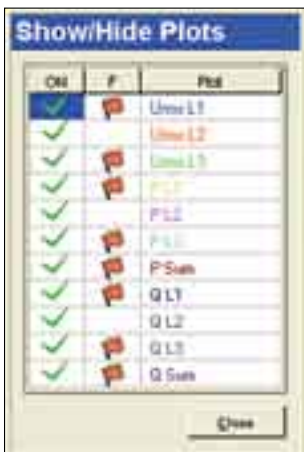
The 1760 provides flagging of data according to IEC 61000-4-30 Class-A. The flagging feature alerts the user that a dip, swell, or interruption occurred during a specific time interval. Values out of nominal ranges are marked by either a colored background or with a flag symbol.
