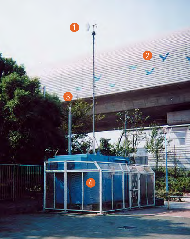
Facility with noise and atmospheric measurement equipment, located next to a highway
