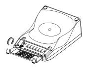
Figure 1: Battery compartment
