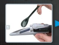
Apply 1-2 drops onto the prism.
