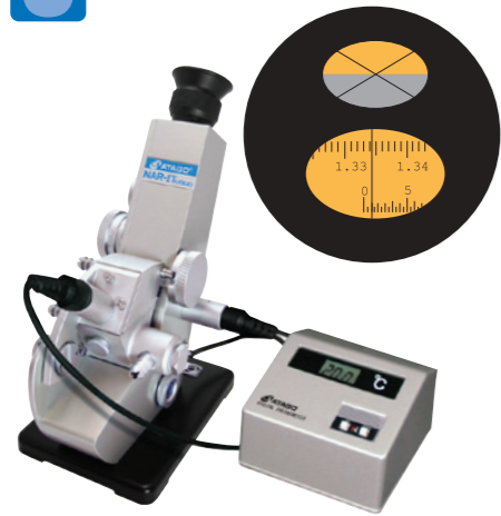
Refractive Index and Brix of liquid samples.
