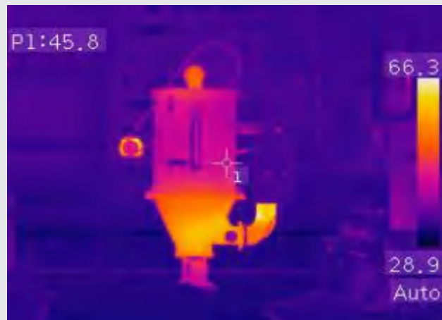
Auto Fusion mode (AUF) A dynamic image enhancement–algorithm for infrared cameras
