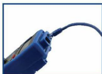
Telephone Line Test(RJ11)
