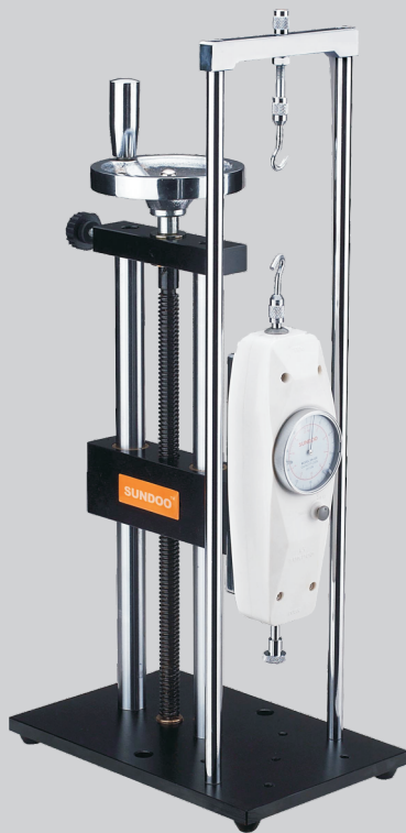
SLJ Wheel manual test stand
