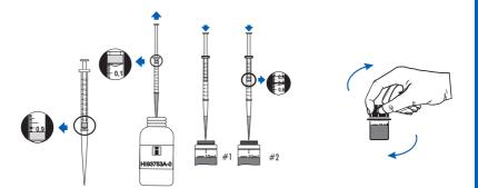
Remove the caps and use the second 1 mL syringe to add 0.5 mL of HI93753B-0 Complexing Reagent to each cuvette.
