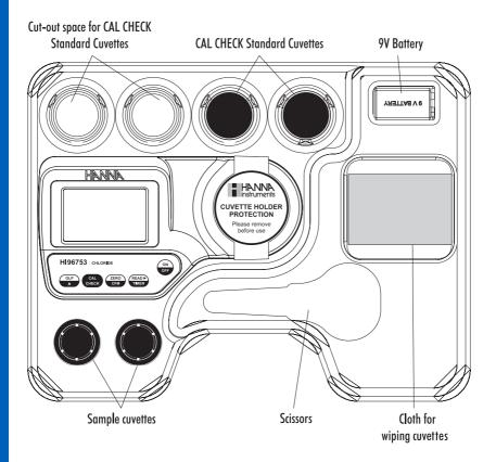
The H196753 is an auto diagnostic portable microprocessor meter that benefits from Hanna Instruments' years of experience as a manufacturer of analytical instruments. It has an advanced optical system based on a special Light Emitting Diode (LED) and a narrow band interference filter that allows most accurate and repeatable readings. All instruments are factory calibrated and the electronic and optical design minimizes the need of frequent calibration.
